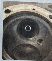
Carbon, carbon everywhere: on the piston crown and throughout the combustion chamber
