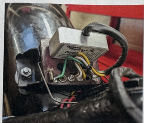
Electronic 6V regulator fitted in the old housing
