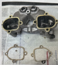
Trying hand cut rocker box gaskets before finding the NOC supplies proper ones
