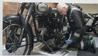
Working on the primary drive
