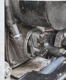
Magneto points secured with a longer, if non-standard 4BA screw. Note the crankcase breather hose
